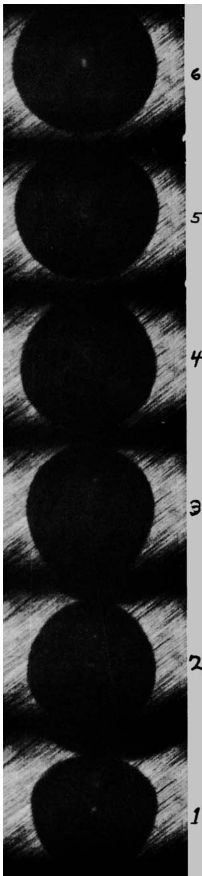
Fig. 7. Microscopic view of pentane bubble vibrating in third mode. The framing rate is 2,520 frames/sec. The field of view is 0.5 mm. high.
